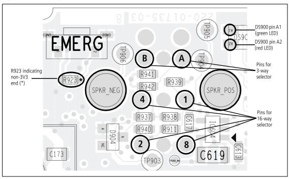
Figure 7.2 PCB layout of pins for RSW1 and DS900 (bottom side)
