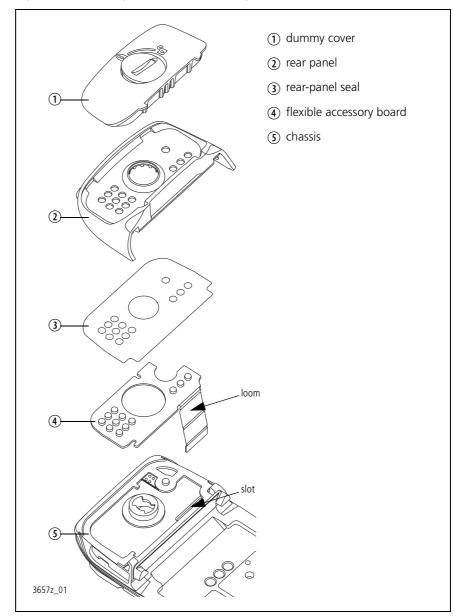
Figure 5.12 Fitting the flexible accessory board and the rear panel
