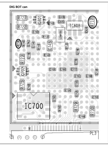
Figure 9.6 Synthesizer components under the DIG BOT can (bottom side)
