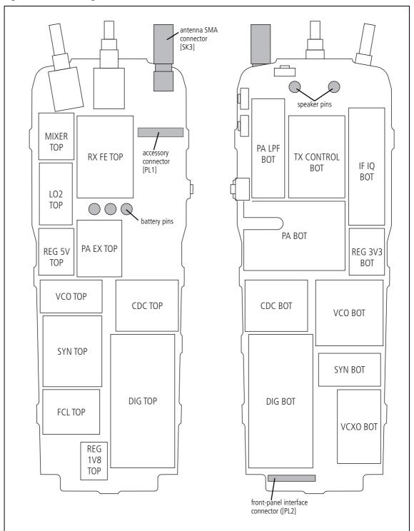
Figure 4.3 Shielding cans and connectors
