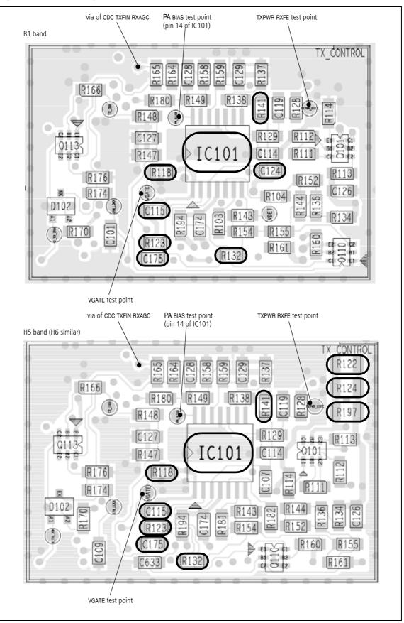
Figure 10.7 PA circuitry under the TX CONTROL BOT can (bottom side)
