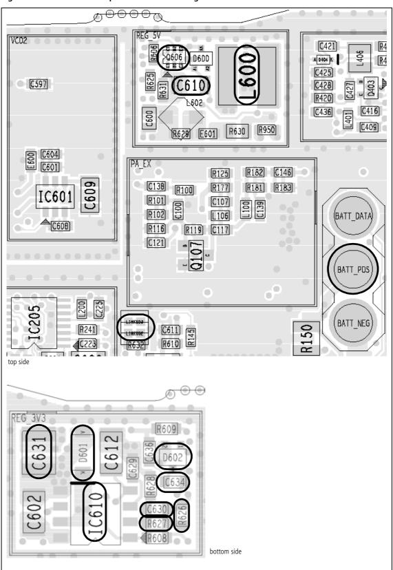
Figure 8.2 Measurement points for the checking the +3V3 SMPS
