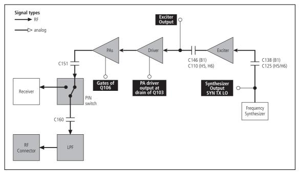
The first point to check in the initial RF signal path is the output SYN TX LO from the frequency synthesizer. This signal is input to the exciter at C138 (B1 band) or C125 (H5, H6).
