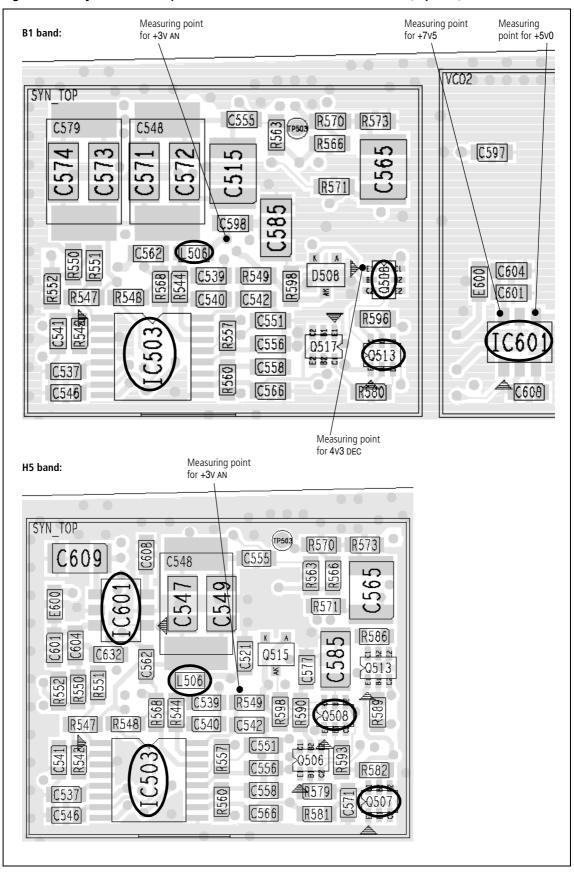
Figure 9.3 Synthesizer components under the SYN TOP and VCO TOP cans (top side)
