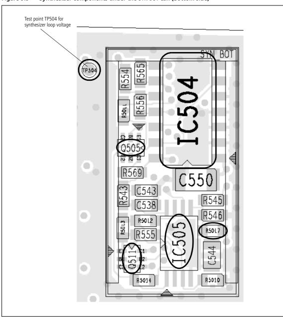
Figure 9.9 Synthesizer components under the SYN BOT can (bottom side)
