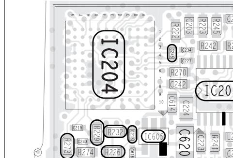
Figure 12.3 Circuitry under and next to the CDC TOP can (top side)
