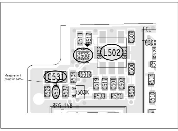
Figure 9.2 Synthesizer 14V power supply circuitry (top side)
