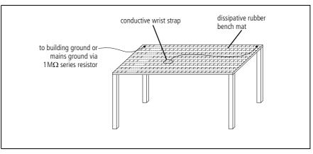
Figure 4.1 Typical antistatic bench set-up
