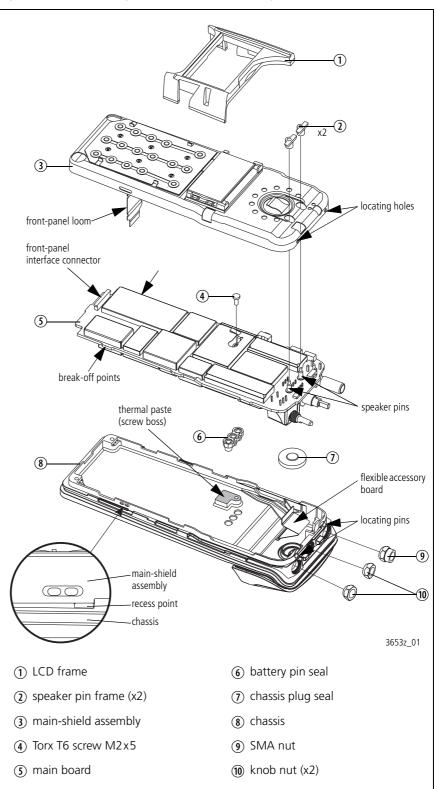
Figure 5.5 Removing the main-shield assembly and the main board
