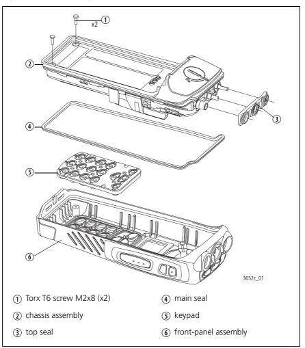
Removing the Main-Shield Assembly The circled numbers in this section refer to the items in Figure 5.5 on page 107.
