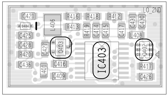
Figure 11.3 Receiver circuitry under the RX FE TOP can (bottom side)
