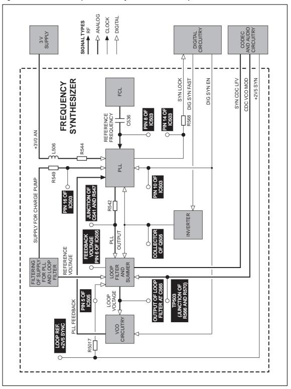
Figure 9.5 Measurement points for the synthesizer PLL and loop filter
