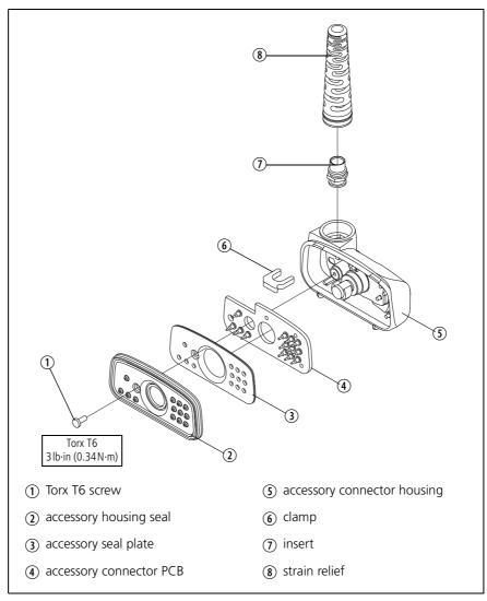
Figure 16.2 Components of the accessory connector kit
