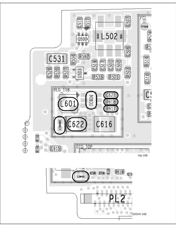
Figure 8.3 Measurement points for the checking the +1V5 SMPS
