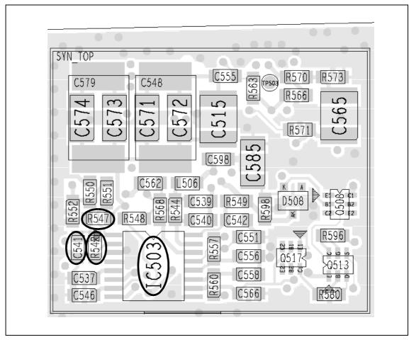
Figure 9.15 Synthesizer components under the SYN TOP can (VHF radio, top side)
