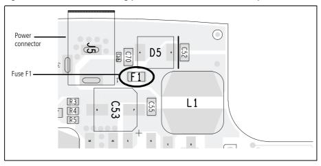
Figure 15.1 Main PCB showing power connector and fuse F1 (top side)
