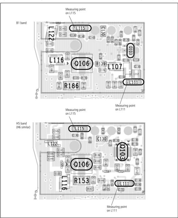
Figure 10.2 Measuring points under the PA bot can (bottom side) for measuring the power supply
